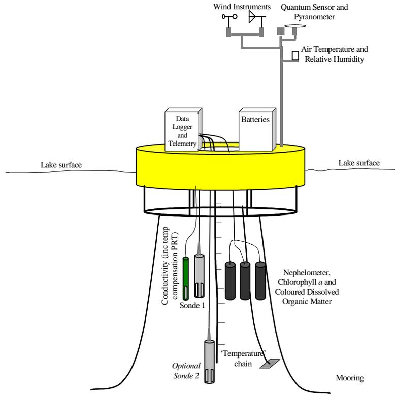
**FIGURE 2** Schematic Diagram of a Lake Dynamics Monitoring Station (LDMS)
