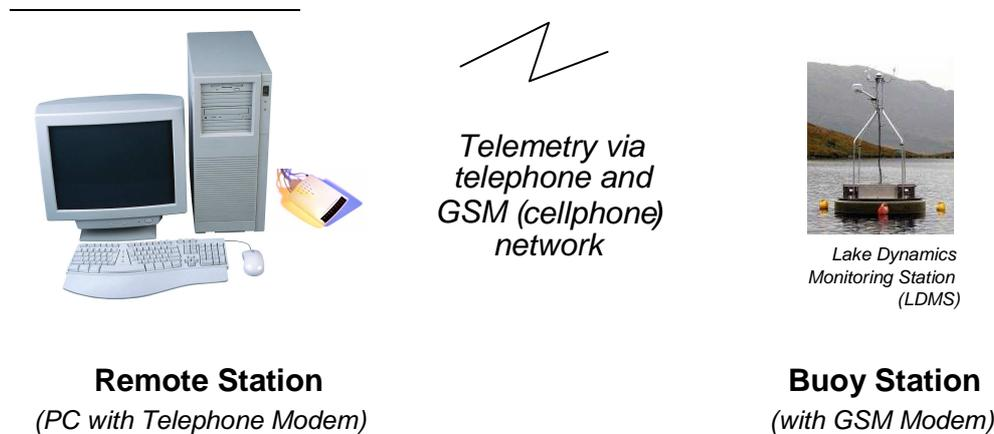
**FIGURE 1** The components of the Lake Dynamics Monitoring Stations
