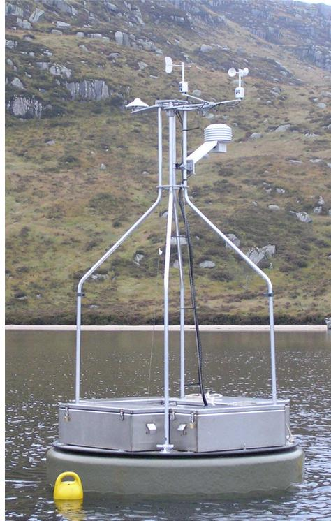
FIGURE 5 a) The deployment of the LDMS at the Round Loch of Glenhead by Helicopter and b) the installed station fitted with the sensors, loggers and communication system..
