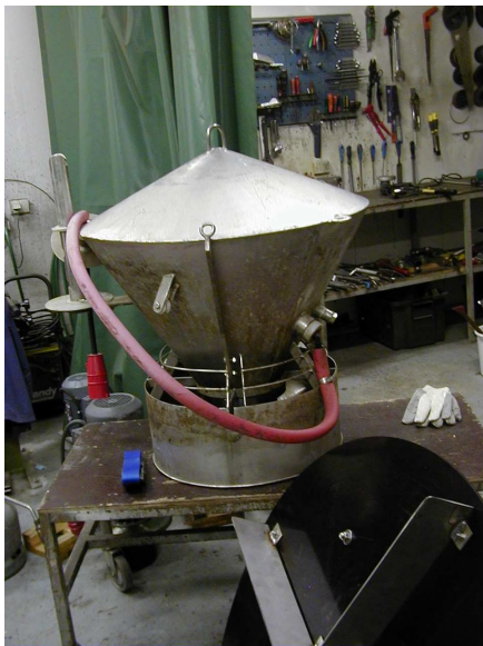
Figure 2. Mixing equipment (MIXOX) used in Lake Halsjärvi.
