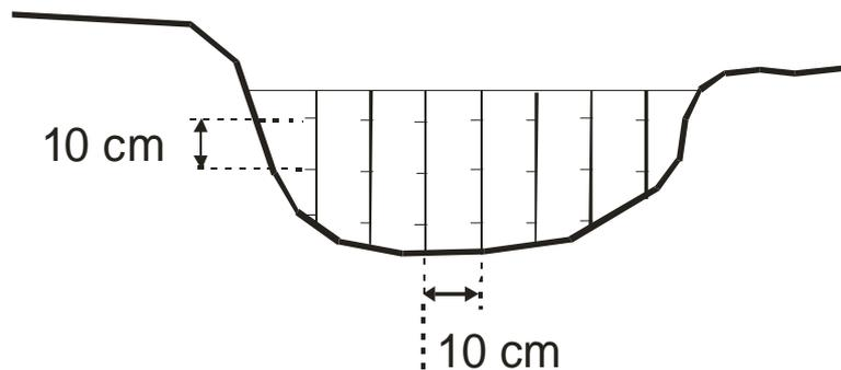
Figure 2. Scheme to measure a current velocity profile.
