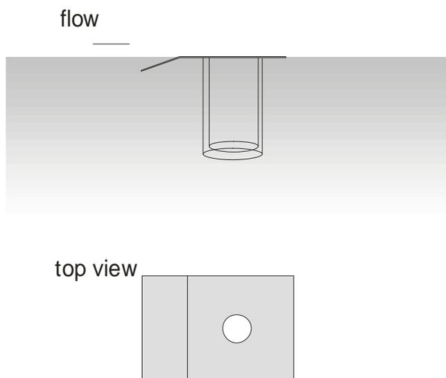
Figure 5. Scheme of the bottom sediment collector.
