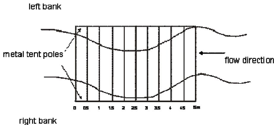
*Figure 4. Example of a grid to map the substrate mosaic on the stream bottom.*
